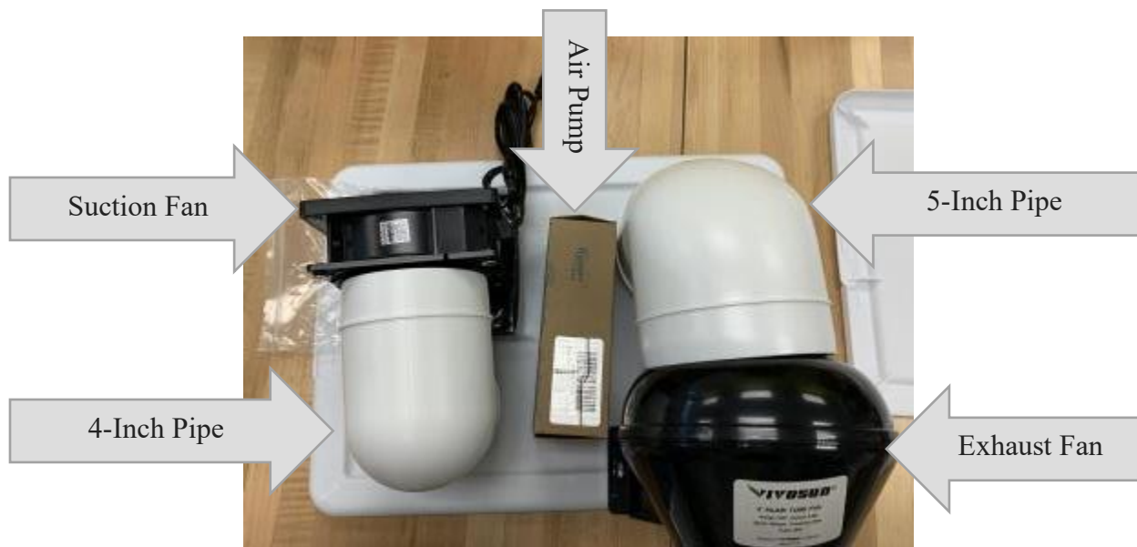
Figure 2: The image above is our tentative setup for the carbon capture device.
