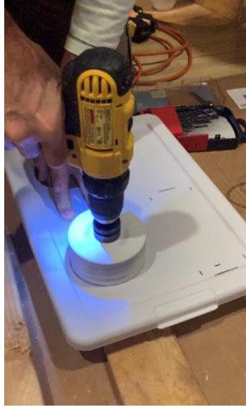
Figure 6: The image above is the drill bit and hole cutter working to cut the hole for the exhaust fan's tube.
