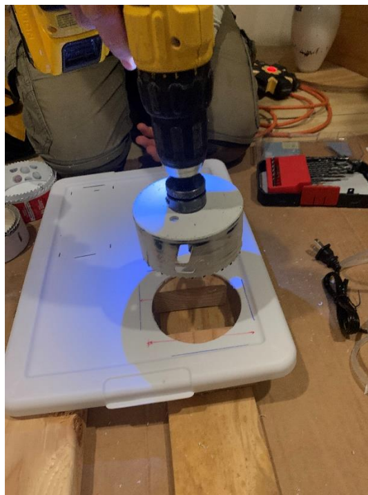
Figure 5: The image above is the drill bit and hole cutter working to cut the hole for the suction fan.
