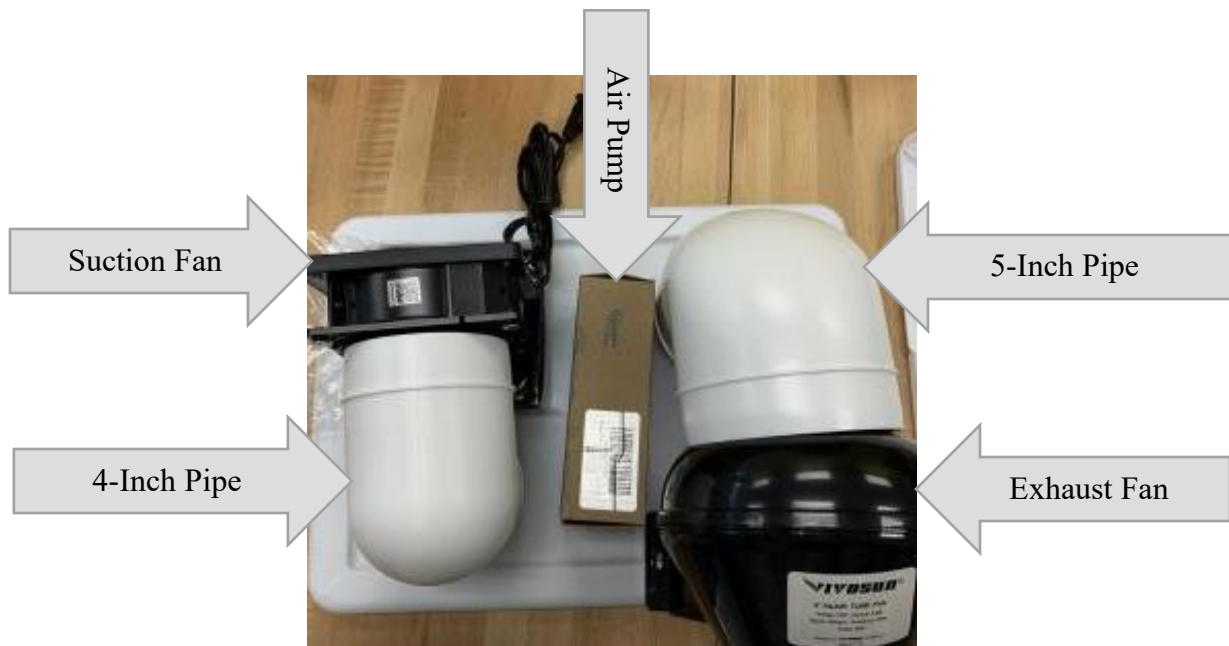
Figure 2: The image above is our tentative setup for the carbon capture device.
